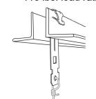
VOH14 pre-tied to #12 GA hanger wire shown attached to the HOIT-AL installation tool on a Lagmaster Plus® telescoping pole tool.
