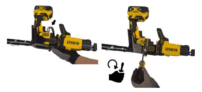
F. Check that the screw gun is parallel to the pole tool and casting. Check both horizontal and vertical alignment of the screw gun. If not aligned properly, repeat step A.
