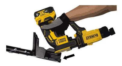
B. Rotate the screw gun until it is level with the casting and slide it all the way in until the grip of the screw gun is pressed up against the grip section of the  $SGP^{TM}$  casting.
